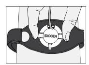
**1.** Squeeze tabs to open the cap on the port.
