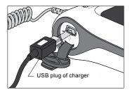
Plug the end of the charger into an electrical outlet. Plug the USB plug end of the charger into the USB port
