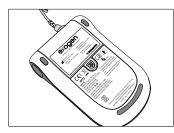
**2.** Turn EXOGEN screen side down and find the battery door screw.
