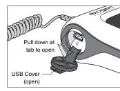
**2.** Pull the tab down to open the USB cover.
