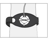
5. Align the cord coming out of the transducer with the notch in the cap. Snap the cap shut on the strap or the cast.
