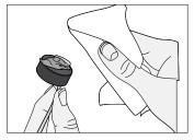
Wipe off any gel on the transducer with a soft cloth. You do not need any cleaning fluid.
