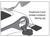
3. Put the Card into the port, metal contacts facing up, and entering first. Press the card into EXOGEN until the card clicks into place.
