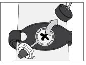
Gently remove the transducer from the port. Do not yank the cord! Pulling hard on the cord to remove the transducer may cause the cord to detach from the transducer and require your EXOGEN to be serviced.
